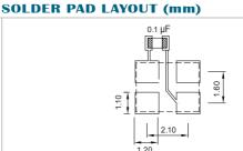
To ensure optimal oscillator performance, place a by-pass capacitor of  $0.1\mu F$  as close to the part as possible between Vdd and GND pads.
