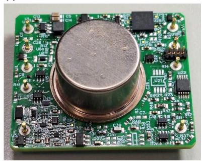
DTQ-100N: Suitable for deployments shorter than 70 days, ideal for shallow waters or lake environments.
